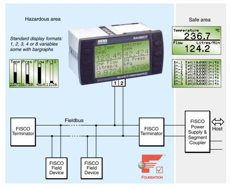
The BA488CF-F Fieldbus Display is an intrinsically safe instrument that can display up to eight fieldbus process variables. Eleven selectable standard screen formats contain one, two, three, four or eight variables, with units of measurement, tag descriptions and bargraphs on some screens.
